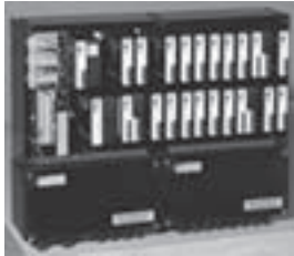
Zone 1 GRP Enclosure with 24 Slots (FB 9224-PG0)
